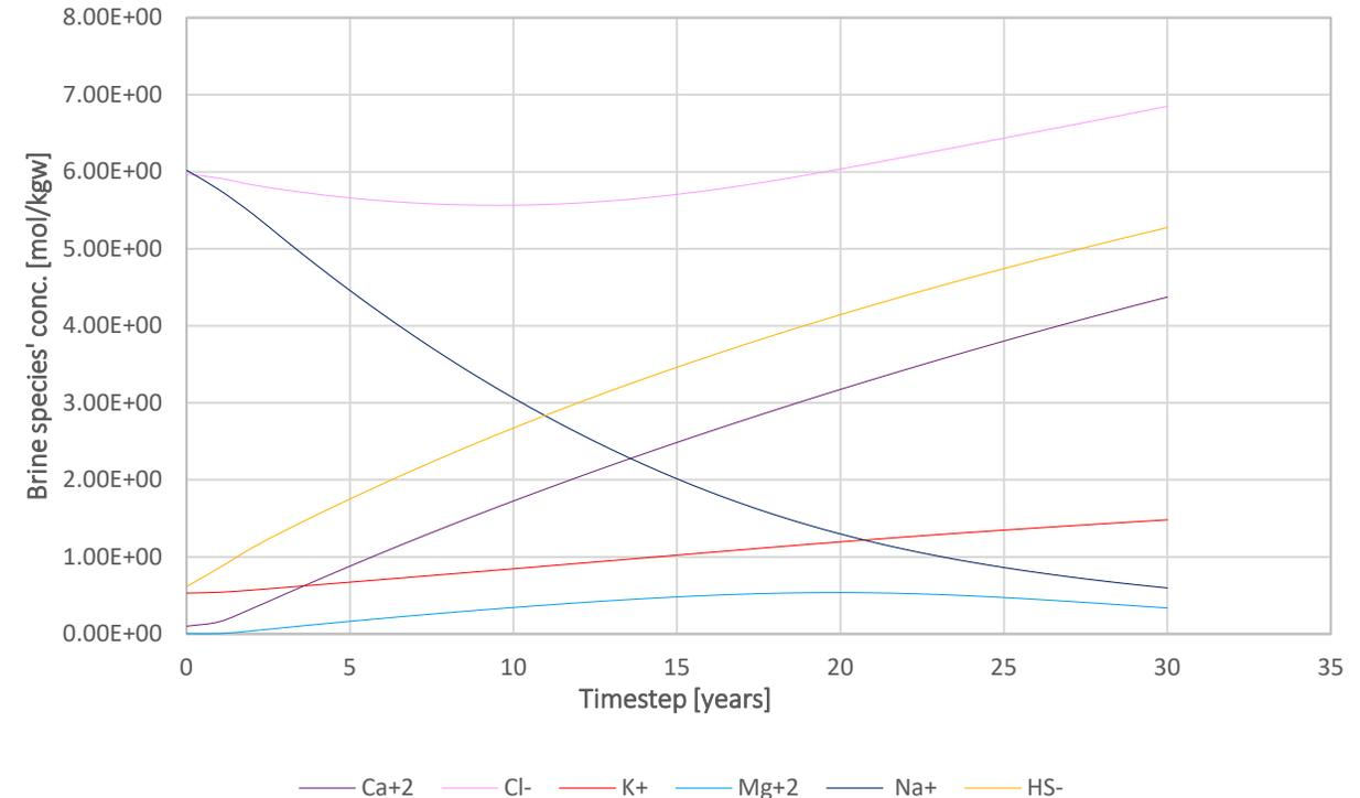
Underground Hydrogen Storage: Distributions and concentrations of Ca<sup>2+</sup>, Cl<sup>-</sup>, K<sup>+</sup>, Mg<sup>2+</sup>, Na<sup>+</sup> and HS<sup>-</sup> in the caprock brine
