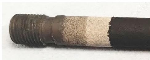
Full cell fabrication (electrolyte and anode layers, anode current collector and sealing)
