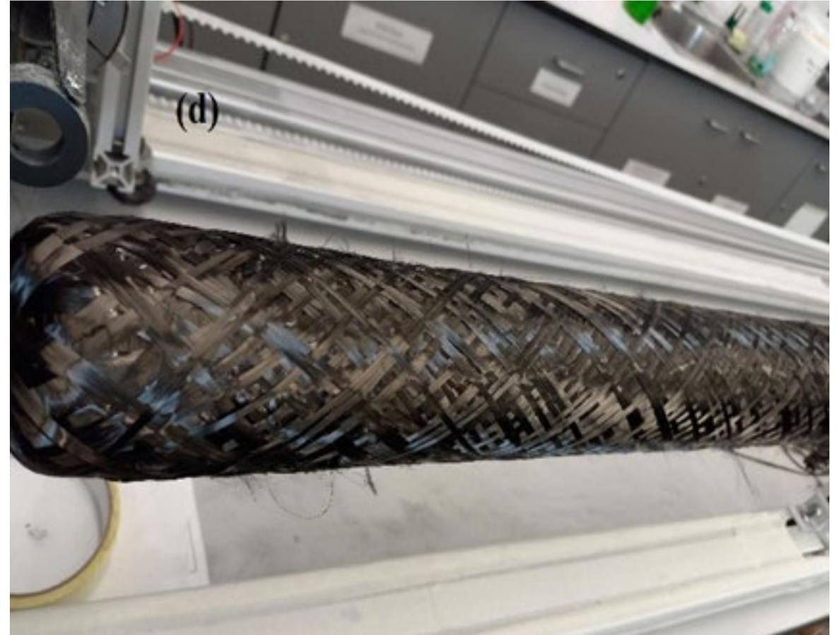
Filament Winding – Composite cylinder manufacturing
