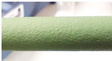
Half cell fabrication (dip coating slurries, current collector & cathode functional layer)
