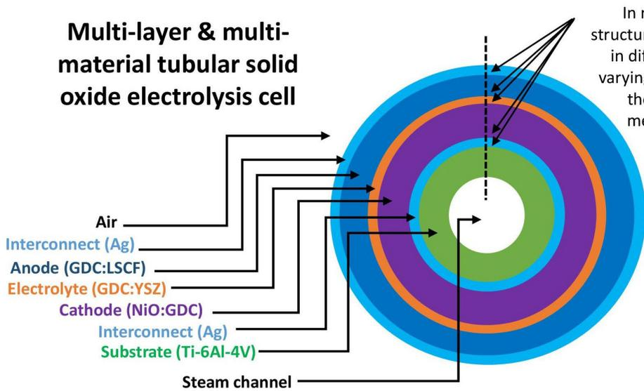
In multi-layer tubular structures, cracks may initiate in different layers due to varying material properties, thermal stresses, or mechanical loading.
