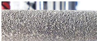
Electrodeposition of silver on SS & Ti tubes
