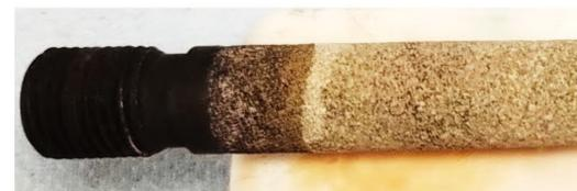
Ultrasonicated slurries, high temperature sintering (950 - 1100 C)
