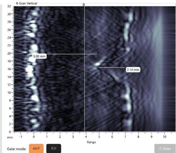
Velocity [m/s]: 5900 Framerate [fps]: 14.6 Applied normalization: Amp:  ToF:
